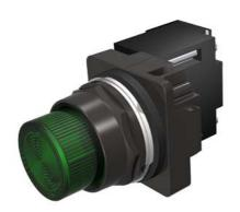
30mm BlackMax, Epoxy Coated Corrosion Resistant Complete Metal Unit Illuminated Indicator Light Transformer type, 600V AC LED Lamp, BA9s Plastic Lens, Green UL Listed, CSA Certified NEMA 1,3,3R,4,4X,12,13 & Automotive Standards
