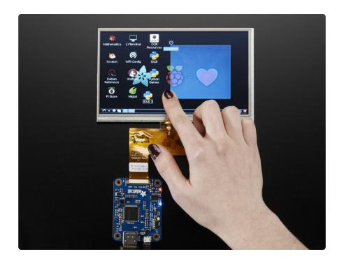
If you purchased the version of the decoder with touch support, you will receive a decoder board with extra circuitry for a resistive touch screen decoder. The circuit is an AR1100 USB resistive touch driver, so it basically just uses the same USB port you use to power, but for the data
