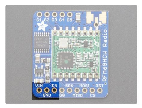
The left-most pins are used for power
