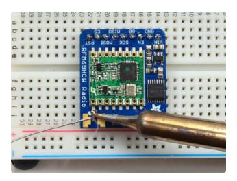
Put down a touch of solder on the signal pad
