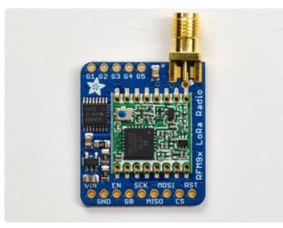
The SMA connector 'slides on' the top of the PCB
