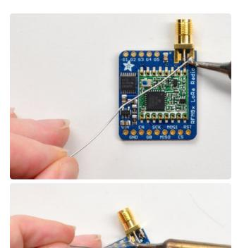
Solder in the two side ground pads. Note you will need a lot of heat for this, because the connector is an excellent heat sink and its got a huge ground plane
