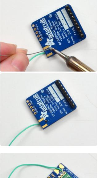
Strip a mm or two off the end of the wire, tin and solder into the **ANT** pad.
