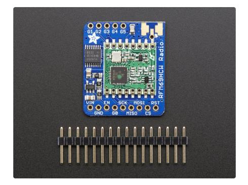
All radios are sold individually and can only talk to radios of the same part number. E.g. RFM69 900 MHz can only talk to RFM69 900 MHz, LoRa 433 MHz can only talk to LoRa 433, etc.
