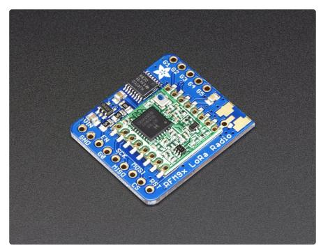
Note that the sub-GHz radio is not designed for streaming audio or video! It's best used for small packets of data. The data rate is adjustbale but its common to stick to
