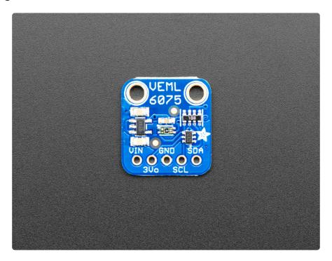
Compared to our other UV sensors, this one actually does a pretty good job of getting accurate UV data. Unlike the Si1145, it has a real UV sensor, and in contrast to the
