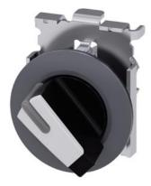
Selector switch, illuminable, 30 mm, round, Metal, matte, white, selector switch, short, front ring for flush installation, 2 switch positions O<I, momentary contact type, Actuating angle 45°, 10:30h/12h, with laser labeling, upper case
