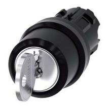
RONIS key-operated switch, 22 mm, round, plastic, lock number SB30, with 2 keys, 3 switch positions I-O-II, latching, actuating angle 2x45°, 10:30h/12h/13:30h, key removal O+I, possible special locks: SB31, 421, 455, with laser labeling, lower case
