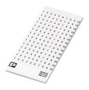
Marker card, Sheet, white, labeled, horizontal: consecutive numbers 1 ... 10, 11 . .. 20, etc. up to 91 ... (99)100, mounting type: adhesive, for terminal block width: 3.81 mm, lettering field size: 3.81 x 2.8 mm, Number of individual labels: 14
