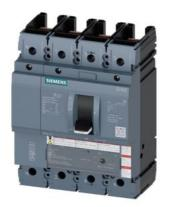
circuit breaker 3VA5 UL frame 250 breaking capacity class M 35kA @ 480 V 4-pole, line protection TM230, FTAM, In=100A overload protection Ir=100A fixed short-circuit protection Ii=5...10 x In N conductor protection 100% without connection
