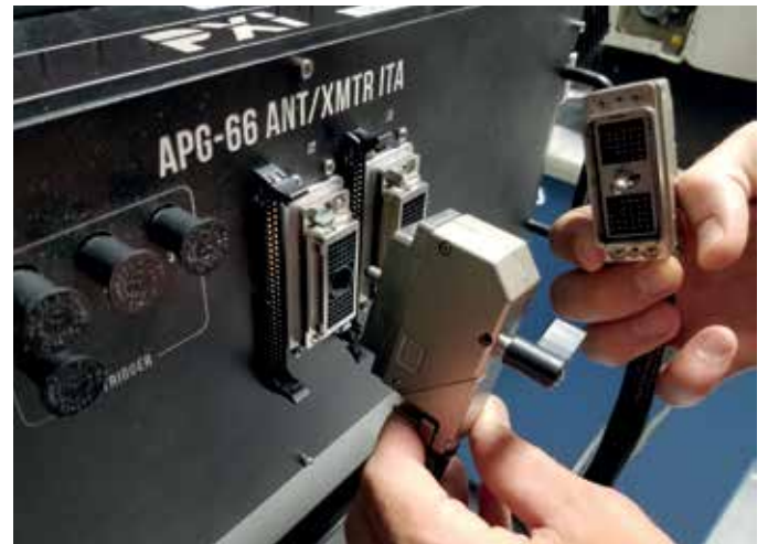
Figure 1: The cam in this test rack is easy to engage with the lever. For tight spaces, the lever can be replaced to move the cam. Another option is a self-actuated cam that, for example can mate and unmate when a drawer is closed or opened. (Learn more at Duotechservices.com )
