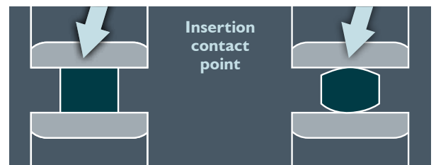
Figure 3: To assume that the use of normal force predicts contact performance is flawed thinking. The domed connector on the right delivers greater reliability because the normal forces are being channeled through a smaller area. Thus, there is more force per unit area available to penetrate the one obstacle standing in the way of stable contact resistance: contact films. (Image: Can Your Connectors Pass the Ultimate Stress Test?)
