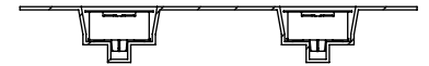
FIG 3 -TR: TAPE & REEL OPTION (MIS-057-01-X-D-K-TR SHOWN) (DIFFERENT AS SHOWN, OTHERWISE SAME AS FIG 1) (-076 POS MAX)
