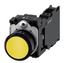
Pushbutton, 22 mm, round, plastic, yellow, pushbutton, flat, momentary contact type, with holder 1 NO+1 NC, spring-type terminal, with laser labeling, inscription or symbol Customer-specific selection with SIRIUS ACT configurator (CIN)
