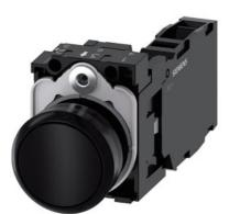
Pushbutton, 22 mm, round, plastic, black, pushbutton, flat, momentary contact type, with holder 1 NO+1 NC, screw terminal, with laser labeling, upper case and lower case, always upper case at beginning of line
