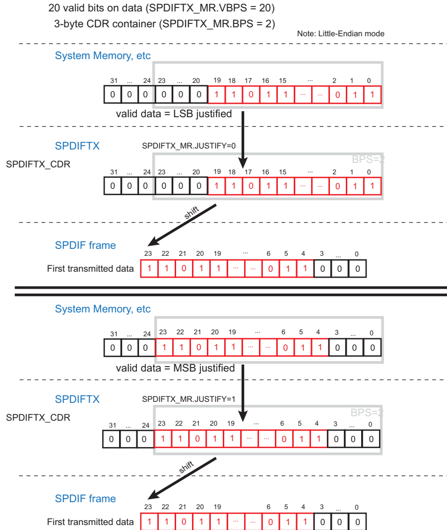
Figure 48-11. Transmitting 24-bit Oriented Data Carrying 20 Valid Bits
