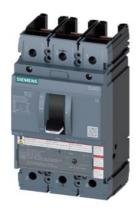
circuit breaker 3VA5 UL frame 250 breaking capacity class H 65kA @ 480V 3-pole, line protection TM230, FTAM, In=150A overload protection Ir=150A fixed short-circuit protection Ii=5...10 x In UL 489 SB (naval),  $50^\circ$  C without connection
