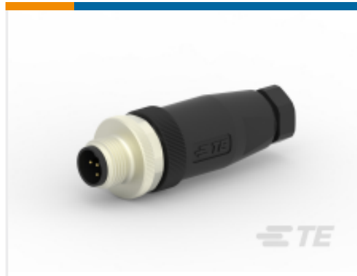
TE Part # T4111401051-000 M12,MALE,STRAIGHT,B CODE,5P, PG7,GOLD
