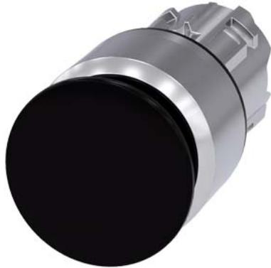
Mushroom pushbutton, 22 mm, round, metal, shiny, black, 30 mm, latching, pull-to-unlatch mechanism, with laser labeling, symbol number according to, ISO 7000 or IEC 60417
