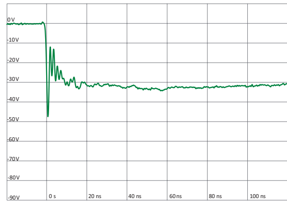
IEC 61000-4-2 -8 kV Contact ESD Clamping Voltage
