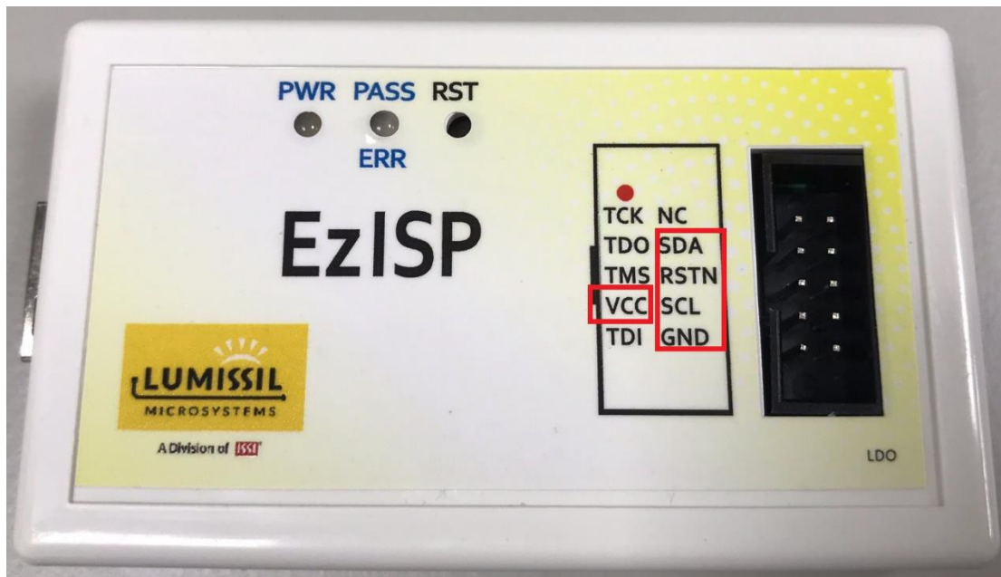
Figure 8-2: Pin configuration on EzISP board
