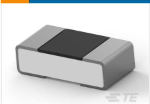
TE Part # 4-2176364-6 RQ 0402 13K7 0.1% 10PPM 5K RL
