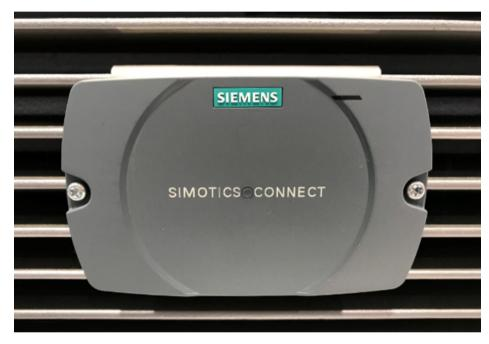
In addition to motor monitoring, from V1.0.2.0, "Generic Vibration monitoring" can be set. Using this function, additional components of the drive train can be monitored, for example, gearbox, coupling, pillow block bearing, pump, fan, compressor as well as other rotating and non-rotating parts.
