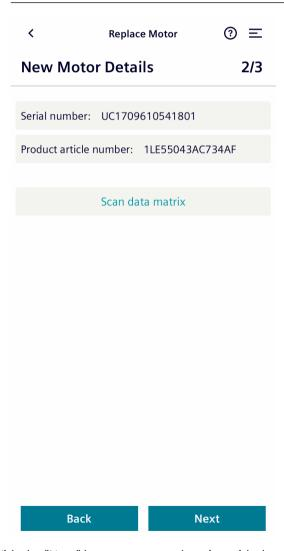
2. With the "Next" button, you synchronize with the cloud. If the motor data set is available in the digital twin database, then you proceed to Step 3/3 - Asset Info.
