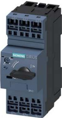
Circuit breaker size S0 for motor protection, CLASS 10 A-release 20...25 A N-release 325 A Spring-type terminal switching capacity 30 kA at 600 V according to UL/CSA
