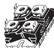
SOT-227[J] Antiparallel Configuration (Isolated Base)
