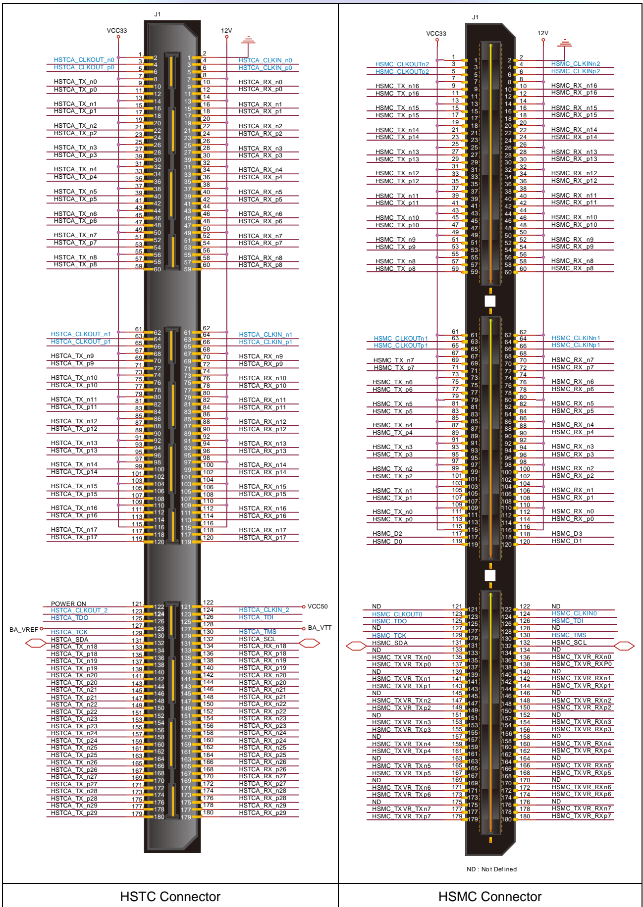
Figure 3.1 The pin-outs of the HSTC and HSMC connector.
