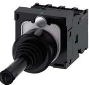
Coordinate switch, 22 mm, round, plastic, black, 4 switch positions, latching, without mechanical interlocking, in O position, with holder, 1 NO, 1 NO, 1 NO, 1 NO, screw terminal, Z=20-unit packaging
