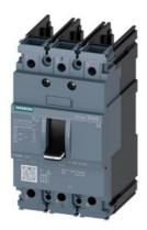
circuit breaker 3VA5 UL frame 125 breaking capacity class H 65kA @ 480V 3-pole, line protection TM210, FTFM, In=100A overload protection Ir=100A fixed short-circuit protection Ii=10 x In UL 489 SB (naval),  $50^\circ$  C without connection
