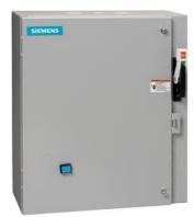
Non-reversing motor starter Size 3 Three phase full voltage Solid-state overload relay OLRelay amp range 25-100A 220-240/440-480VAC 60HZ coil Combination type 125Amp circuit breaker Enclosure NEMA type 1 Indoor general purpose use Standard width enclosure
