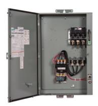
Pump control panel, Size 4, Three phase full voltage, Solid-state overload relay, OLR amp range 50-200A, 24VAC 50-60Hz coil, Standard type contactor, 200A fusible disconnect, 200A/250V fuse clip, HOA Sel Sw. <(>&<)> Start P.B., Enclosure NEMA type 3/3R, Weather proof outdoor use
