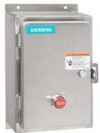
Non-reversing motor starter, Size 2, Three phase full voltage, Solid-state overload relay, OLR amp range 13-52A, 110V 50Hz / 120V 60Hz coil, Non-combination type, Encl. type 4X 304 S. Steel, Water/dust tight noncorrosive, Standard width enclosure
