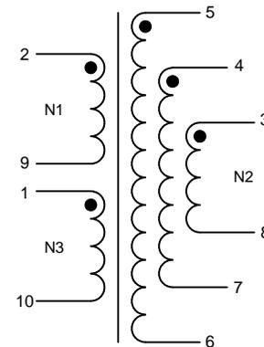
N2 denotes three windings connected in parallel. Terminals 3+4+5 and 6+7+8 must be tied as solder bridging is allowed.
