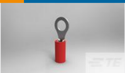
TE Part # 32837-1 TERMINAL,PIDG R 22-16 10
