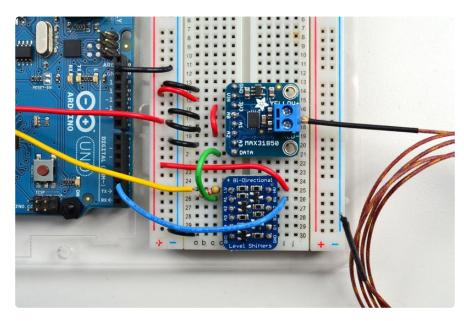
Now if you open up the serial console you should see the OneWire example code print out the data, address and temperature of the sensor. If you mess with the **Ax** wires you'll see this address value change from 0x00 to 0x0F. This can be a good way to deal with 'hot-swapping' in sensors with unique ROM addresses
