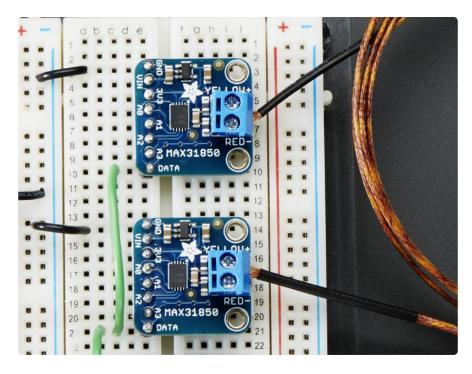
The MAX31850K data format is very similar to that of the well known 1-Wire DS18B20 temp sensor but it is not drop in compatible without code changes to check for the new '1 Wire family' type. We have adapted the classic Arduino <u>OneWire (https://adafru.it/dal)</u> and <u>DallasTemp (https://adafru.it/dam)</u> libraries to be MAX31850 compatible, so please click on those links to grab our libraries.
