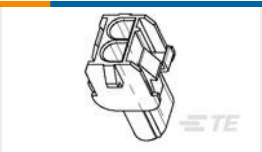
TE Part # 1-1703062-2 CAP, 2 CIRCUIT, UNIVERSAL MATE-N-LOK
