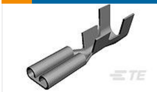
TE Part # 41449 250 FASTON REC 14-10 AWG BR
