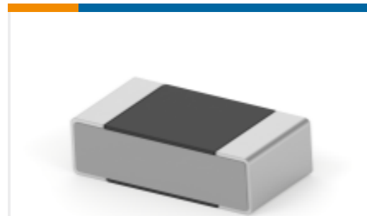
TE Part # 7-1879140-6 RN 0603 113K 0.1% 10PPM 5K RL
