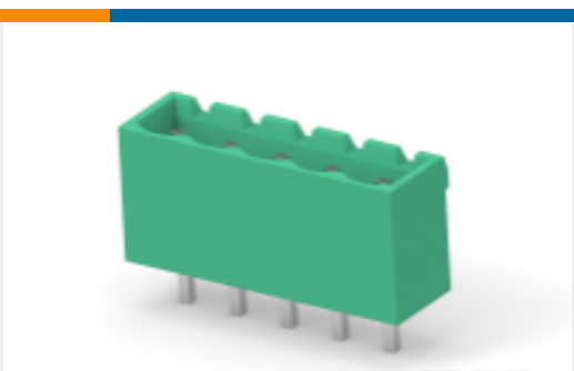
TE Part # 2351885-5 5POS TB HDR 180 DEG, PITCH 5.0&TL 4.5mm
