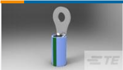
TE Part # 134122-1 TERM, PIDG, R, IR, 14, M5
