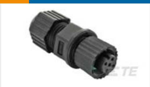
TE Part # 1838274-2 M12 Fld Ser CONN. Female Skt Sldr
