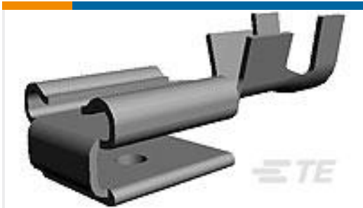
TE Part #61944-2 250 FASTON REC 18-14 AWG TPBR
