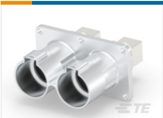
TE Part #2413971-2 HD1400 2PIN 180DEG BB CODE NO HVIL TOP
