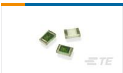
TE Part # 7-2176089-2 RP 1J 0.166W 63K4 0.1% 25PPM 1K RL
