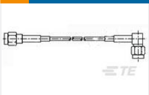
TE Part # 1337810-2 50 OHM COAX SMA STR PLUG ELB P SW
