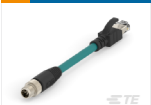
TE Part # TCX3872A202-004 M12 X-code 8pin Male to RJ45 Cable Assembly, Cat6A TPE 26AWG Shielded
