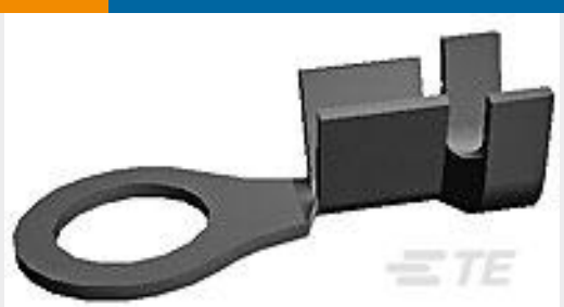
TE Part # 40951 RING 18-14 AWG .0198 X .343 BR
