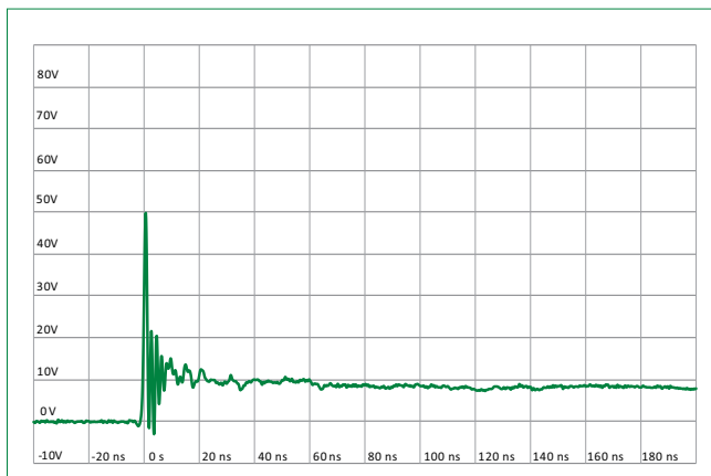
IEC 61000-4-2 +8 kV Contact ESD Clamping Voltage
