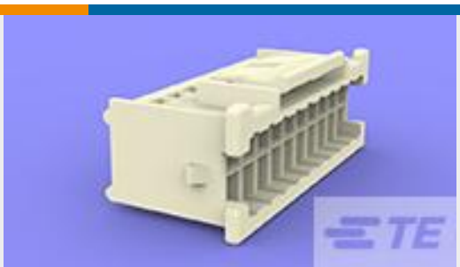
TE Part # 280373-2 8P AMPMODU II SHRD HDR, ST, 0.38 AU
