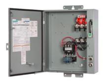
Pump control panel, Size 2, Three phase full voltage, Solid-state overload relay, OLR amp range 13-52A, 220-240/440-480VAC 60Hz coil, Standard type contactor, 60A fusible disconnect, 60A/250V fuse clip, HOA Sel Sw. <(>&<)> Start P.B., Enclosure NEMA type 3/3R, Weather proof outdoor use
