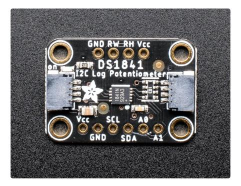
Potentiometers are the perfect tool when you want to change your circuit by turning a knob. Turns out, there are times when you want to adjust your circuit without manually turning a knob, and the **DS1841 I2C Logarithmic Resistor from Maxim** can do just that. It's a programmable resistor, similar to an I2C potentiometer like the the **DS3502 I2C**Potentiometer (http://adafru.it/4286), so why another?
