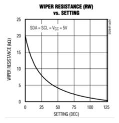
This graph shows the relationship between the wiper setting and the resulting resistance. At the start, the changes are relatively large, but as the values increase, the resulting change in resistance gets smaller and smaller.
