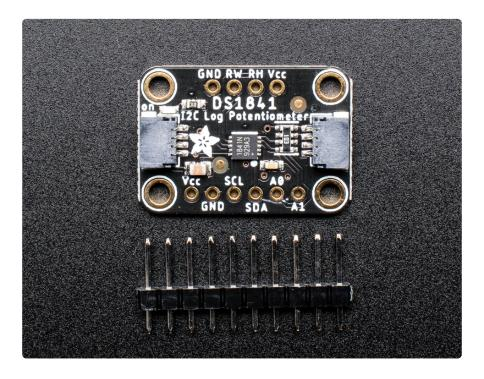
Working with the DS1841 is easy. We've put it on a breakout PCB with the required support circuitry and SparkFun qwiic (https://adafru.it/Fpw) compatible STEMMA
