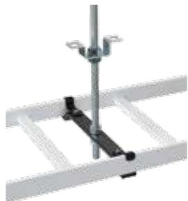
Threaded rod and bracket supports center of ladder rack from ceiling. Kit includes heavy-duty ladder rack cross member, two mounting brackets, two #12-24 screws, 5/8-in. threaded rod, protected sleeve and four 5/8-in. nuts. Use one kit at least every 5 ft. (1.5 m). Made of plated steel.
