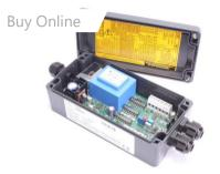
Load Cell Amplifier | Load Cell Signal Conditioner | SGA Inputs from 0.06mV/V From £211
