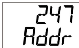
Screen No. 2: Modbus address
